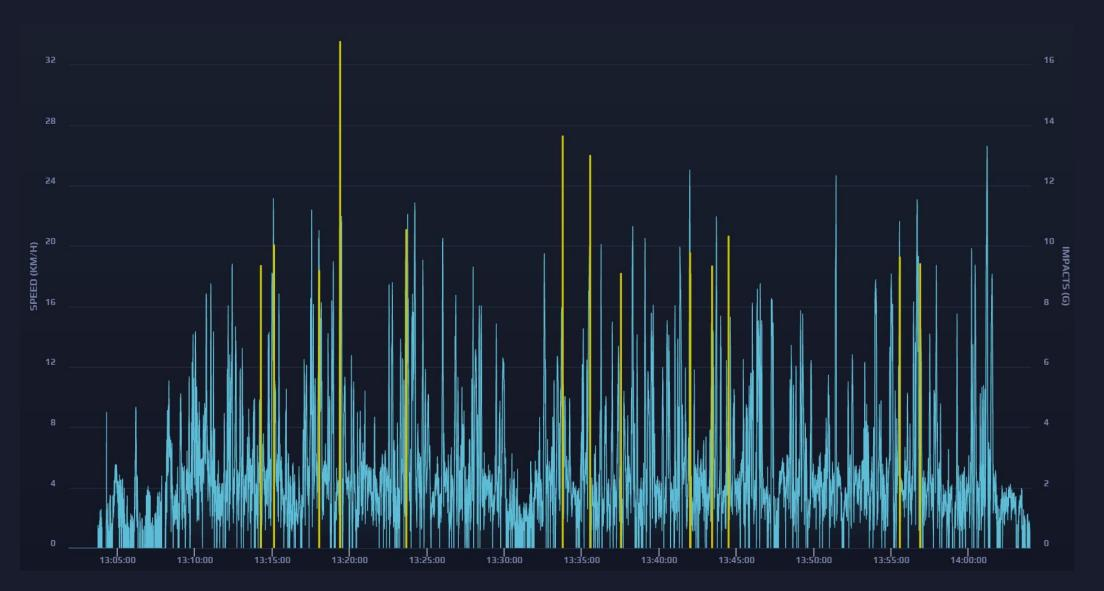
Measured in G-force using accelerometer data to provide a count, based on zone criteria. Impacts can vary from a wide range of areas including weighted impacts, collisions, tackles, ball strikes, etc. As a player becomes more fatigued it is common to notice impacts increase due to the foot striking the ground harder during a run.
