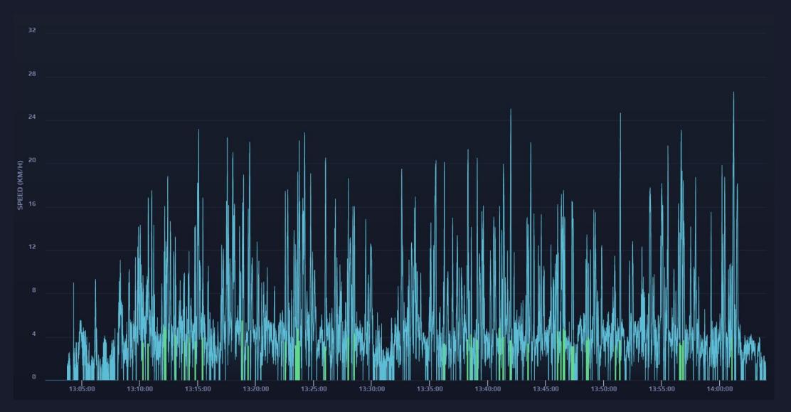
Number of accelerations performed in a session or game. An acceleration is defined as a change in speed with a magnitude of 3 m/s<sup>2</sup> or above and must be maintained for at least half a second. In terms of running, anytime the body starts, speeds up, or changes direction, it is accelerating.
